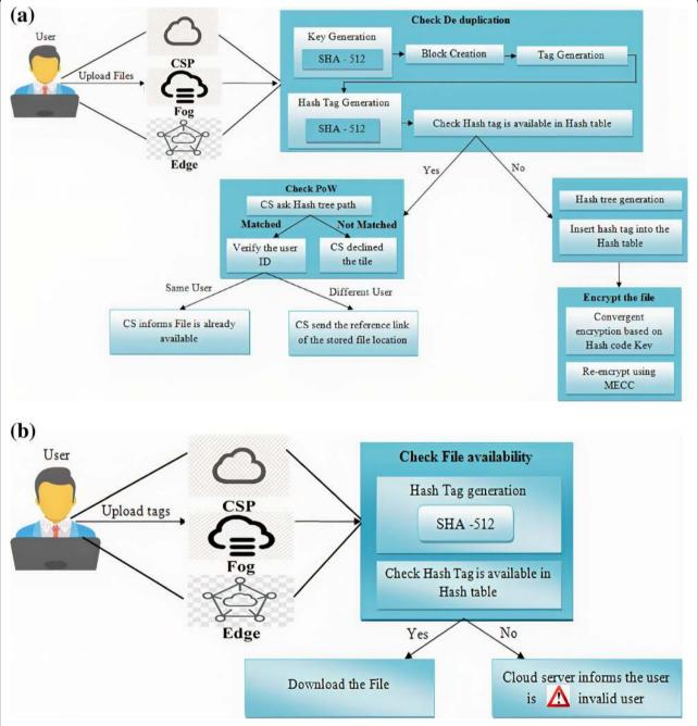
Fig. 1 a Uploading the file into the cloud server using the proposed system. b Downloading the file from the cloud server using the proposed system
