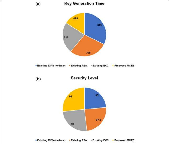
Fig. 4 a Performance comparison of proposed MECC with existing techniques in terms of key generation time. b Performance comparison of proposed MECC with existing techniques in terms of security level
