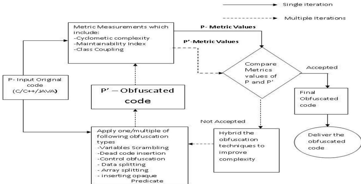
Figure1 Propose Block diagram – M-COT (Metrics based Code Obfuscation Techniques)
