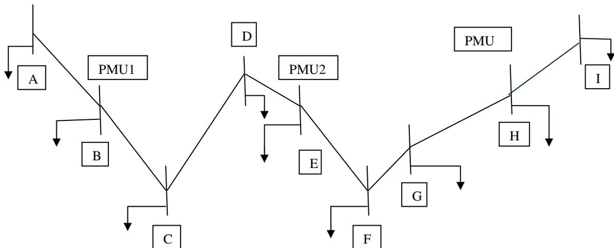
Figure 1. Complete observability using PMU's
