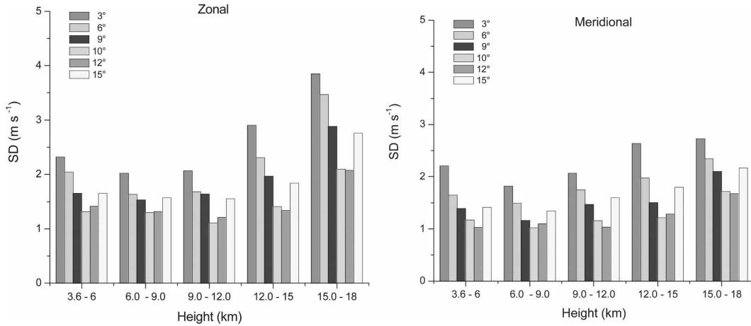
FIG. 1. SD differences in wind velocities between the GPS sonde and the radar observations for different tilt angles.
