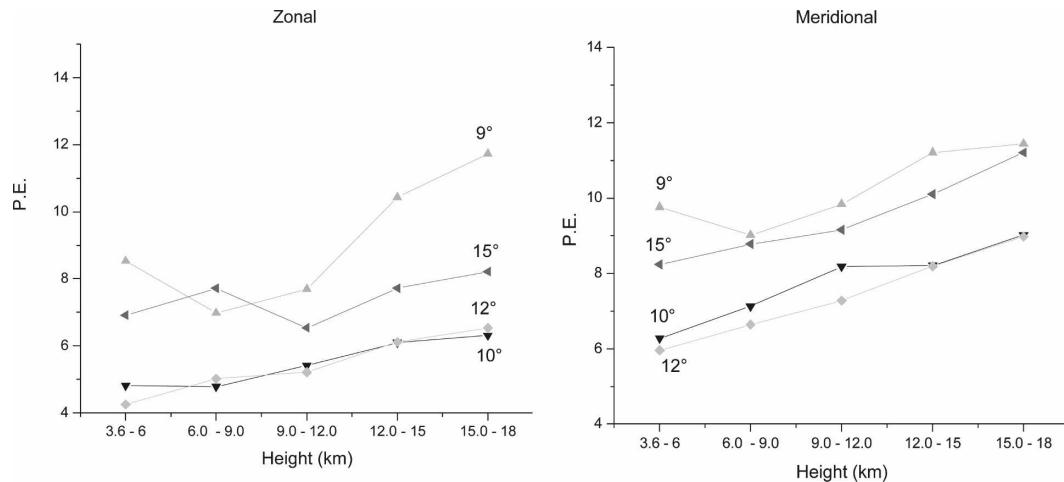
FIG. 10. PE in horizontal wind velocities after effective beam angle correction.
