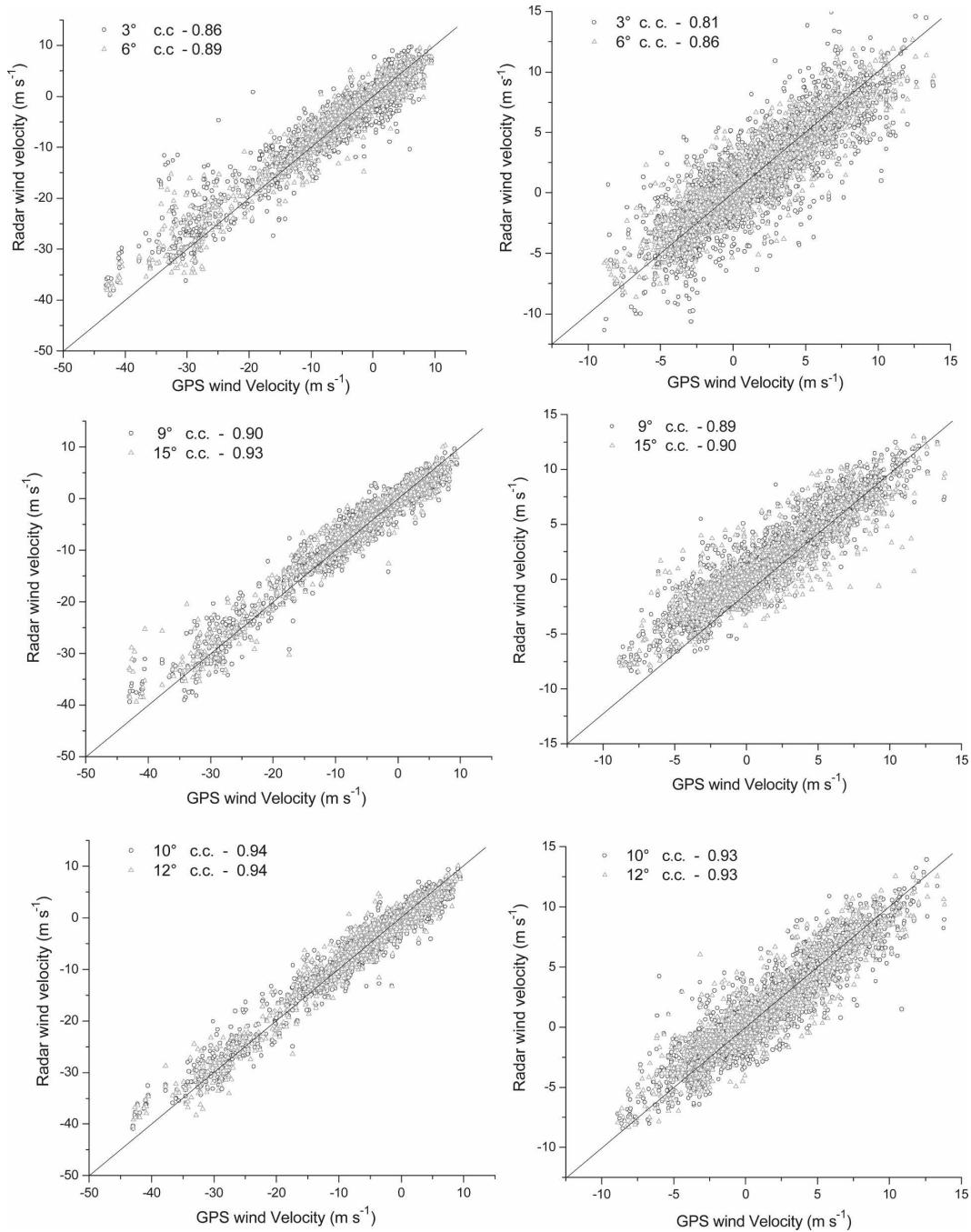
FIG. 3. Scatterplots of the GPS sonde vs the radar measurements for different tilt angles from a height range of 3.6–18 km. (left) Zonal velocity and (right) meridional velocity.
