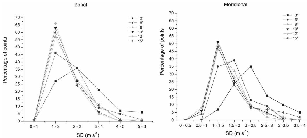
FIG. 2. Percentage of data points having SD differences in the horizontal wind velocities between GPS sonde and radar measurements with an interval of 1 m s<sup>-1</sup> for the zonal component and 0.5 m s<sup>-1</sup> for the meridional component.
