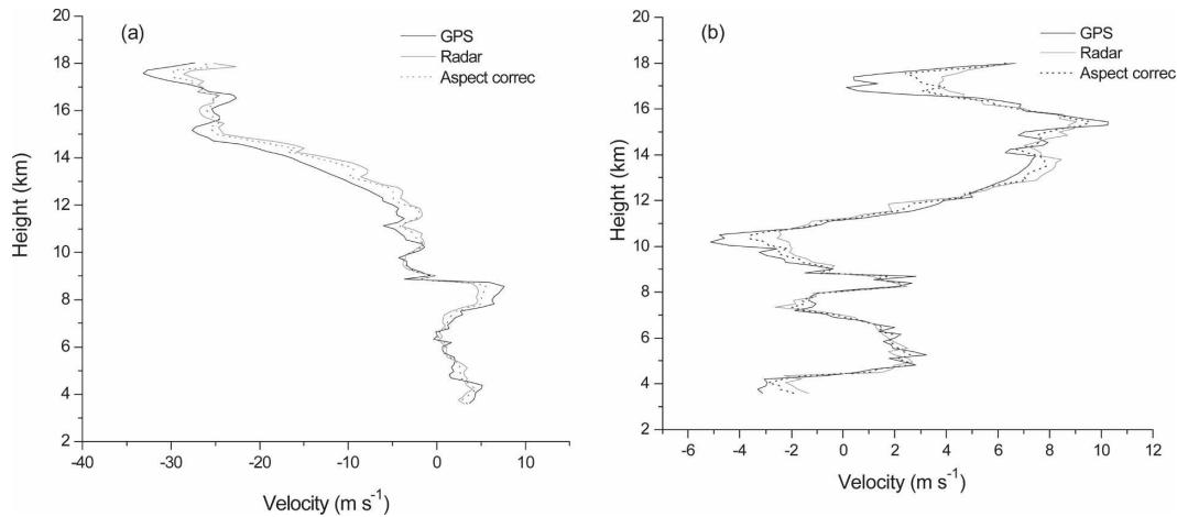
FIG. 8. Vertical profiles of horizontal velocities: (a) zonal and (b) meridional observed with GPS sonde (solid black), radar (solid red), and aspect corrected radar (dotted blue) on 25 Sep 2002.
