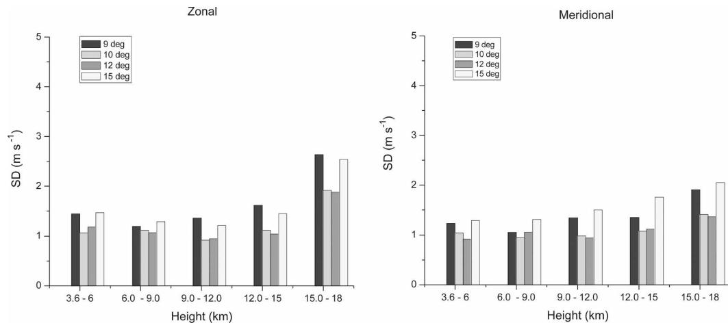
FIG. 9. SD differences in wind velocities between the GPS sonde and the radar observations for different tilt angles after effective beam angle correction.
