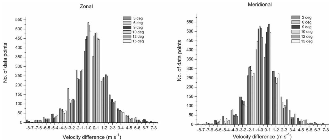
FIG. 4. Horizontal wind velocity differences between GPS sonde and radar plotted with an interval of 1 m s<sup>-1</sup>.
