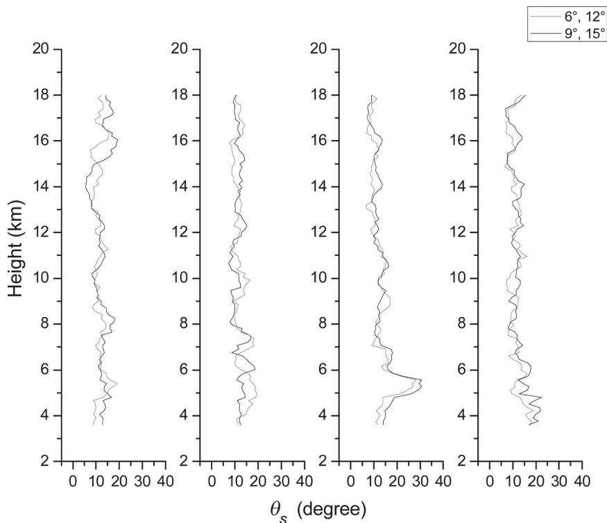
FIG. 7. Height profiles of  $\theta_s$  for various beam combinations observed on 25, 26, 28 Sep and 9 Oct 2002 in east-west plane.
