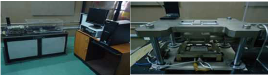
Fig.1.(a)the experimental setup (b)close view of the upper and lower specimen holders
