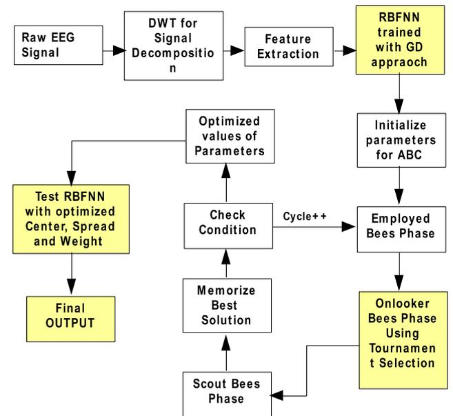
**Figure 7** Model of classification using RBFNNN with ABC algorithm.
