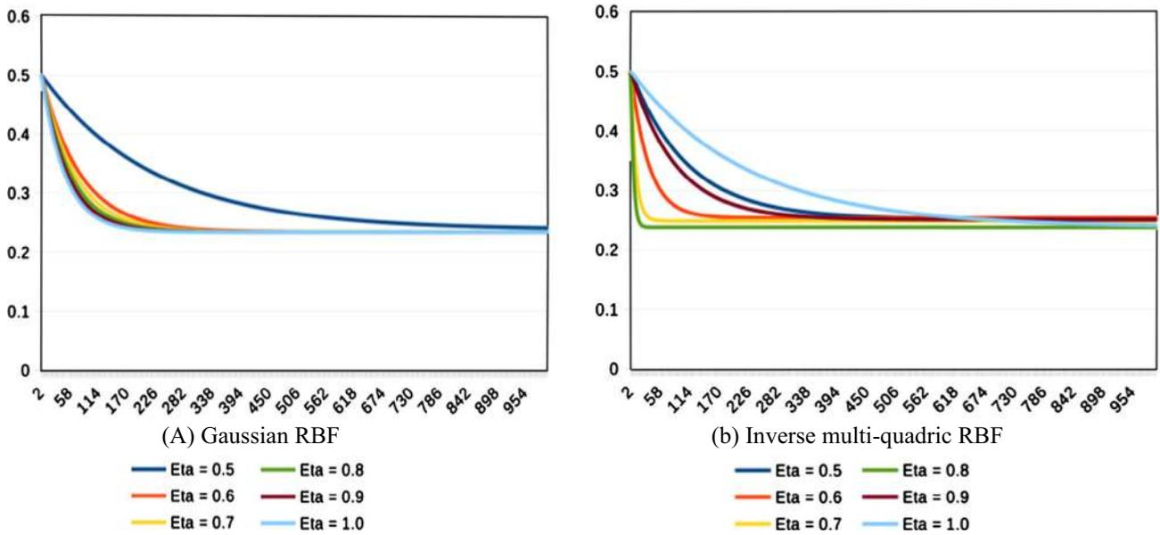
Figure 8 Experiment 1 (A & E) MSE graph for gradient descent approach with varying  $\eta$  value.
