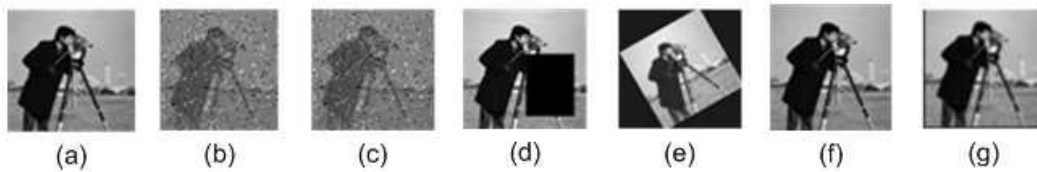
Fig. 7. Retrieved watermarks with (a) No attack (b) salt and pepper noise (c) Gaussian noise (d) cropping (e) rotation (f) scaling and (g) translate Attacks
