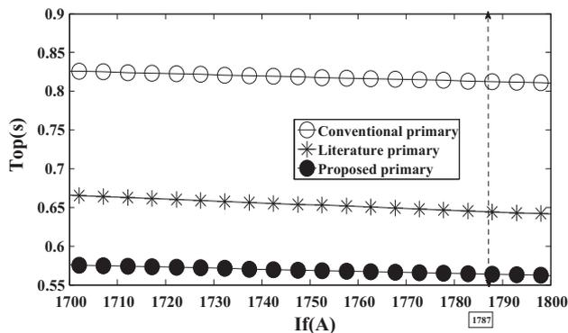
Fig. 5. Working time features of Re.48 in IEEE 30 bus distribution electrical test system.
