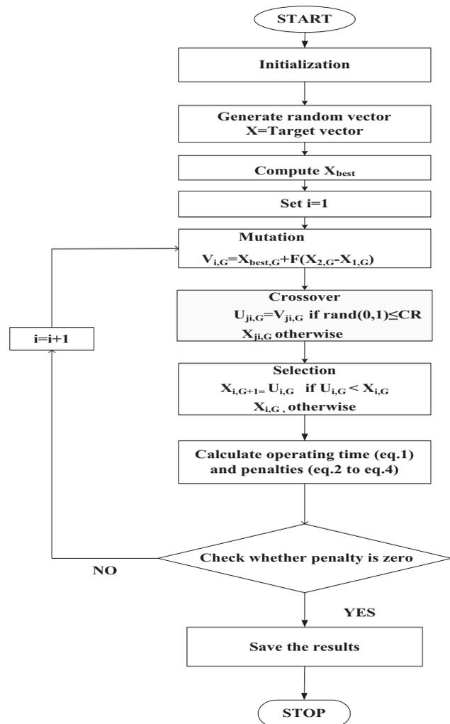
**Fig. 1.** Flow chart of relay in-service time calculation.
