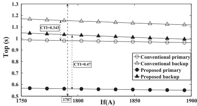
Fig. 4. Functioning time features of Re.48 and Re.52 in IEEE 30 bus electrical distribution test system.
