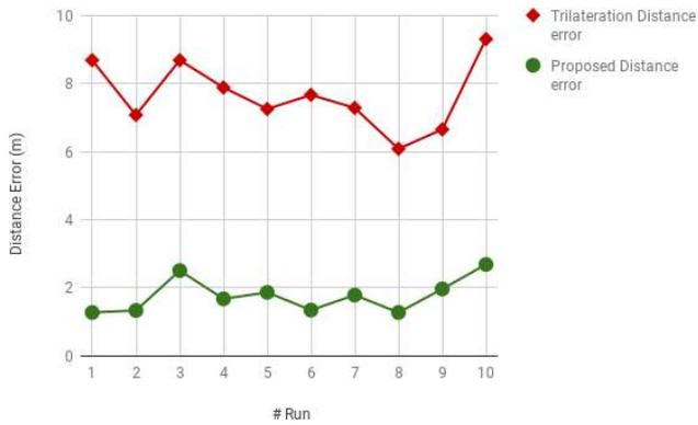
**Figure 8:** Distance Error by Trilateration and PHA-IPS method
