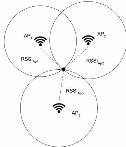
Figure 1: Wi-Fi Trilateration using RSSI measured method
