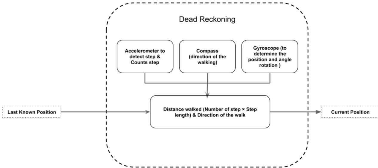
Figure 3: Position estimation with the inertial sensors of a smartphone
