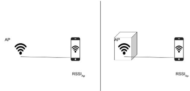
Figure 5: RSSI signal at a distance without & with block in the direct path
