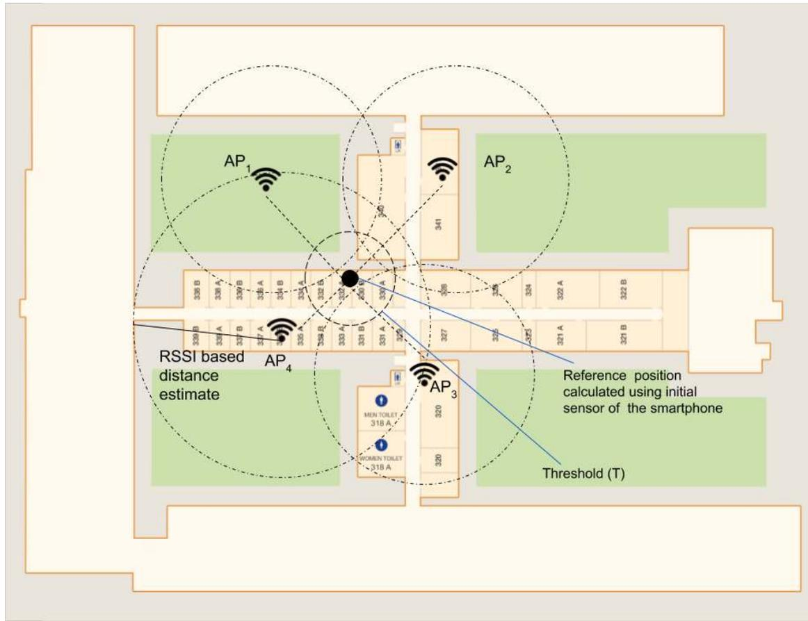
Figure 7: Position estimate by avoiding the anomaly nodes in the system
