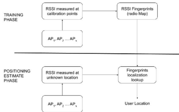
Figure 2: Wi-Fi Fingerprinting positioning estimation method
