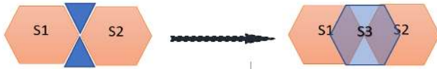
Fig. 9. Optimum Sensor node s3 estimation and deployment between s1 and s2 to cover the weak zone area
