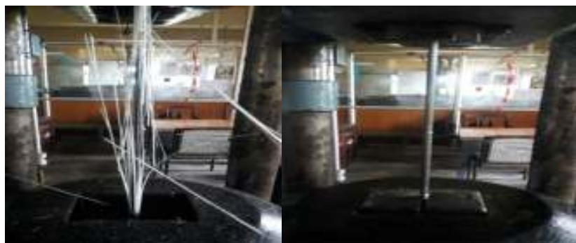
Figure 3. Test set up and rupture of rebars
