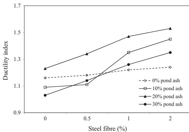
**Figure 13** Effect of steel fibre on ductility index.
