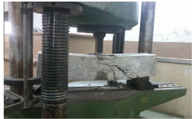
Figure 8 Failure pattern of beam specimen.
