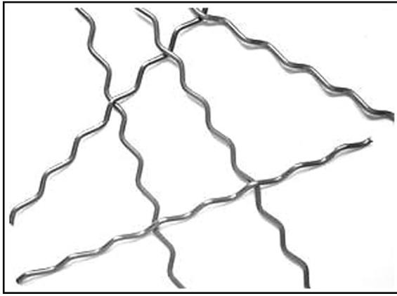
Figure 3 Grooved steel fibres.
