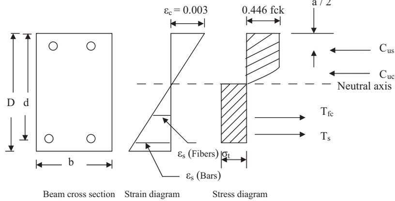
Figure 5 Stress strain diagram of beam section.
