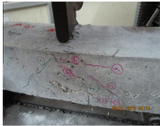
Figure 7 Formation of cracks for A4 beam specimen.
