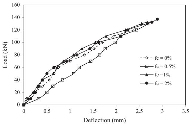
**Figure 12** Load vs mid-span deflection of fibre reinforced concrete beam (30% pond ash).
