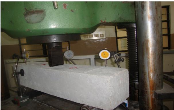
Figure 6 Testing of beam under universal testing machine.
