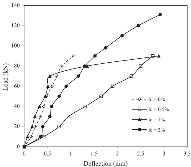
Figure 9 Load vs mid-span deflection of fibre reinforced concrete beam (0% pond ash).
