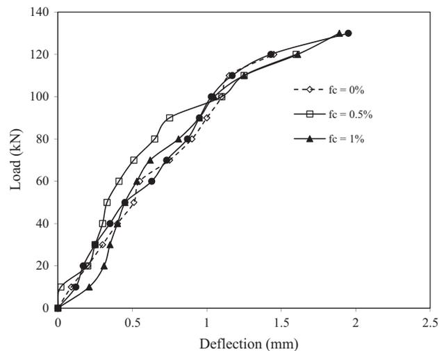
Figure 11 Load vs mid-span deflection of fibre reinforced concrete beam (20% pond ash).
