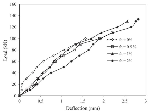
Figure 10 Load vs mid-span deflection of fibre reinforced concrete beam (10% pond ash).
