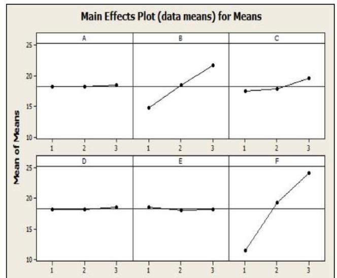
**Fig. 6.** Main effect plot of Surface roughness.
