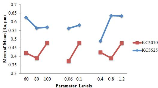
**Figure 2.** Main effect plots for surface roughness (Ra) for KC5010 and KC5525.
