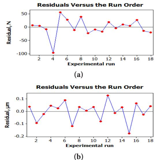
**Figure 4.** Residuals versus experimental run: a) cutting force (KC5525); b) surface roughness (KC5525).
