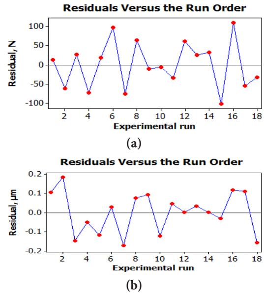
**Figure 3.** Residuals versus experimental run: a) cutting force (KC5010); b) surface roughness (KC5010).
