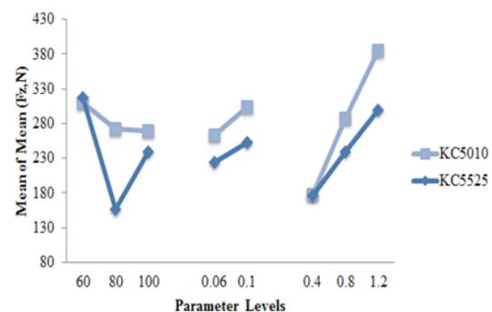
**Figure 1.** Main effect plots for mean of mean for cutting force (Fz) for KC5010 and KC5525.
