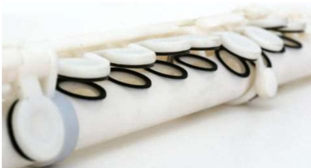
Fig. 4 Additive-manufactured flute. Source [20]
