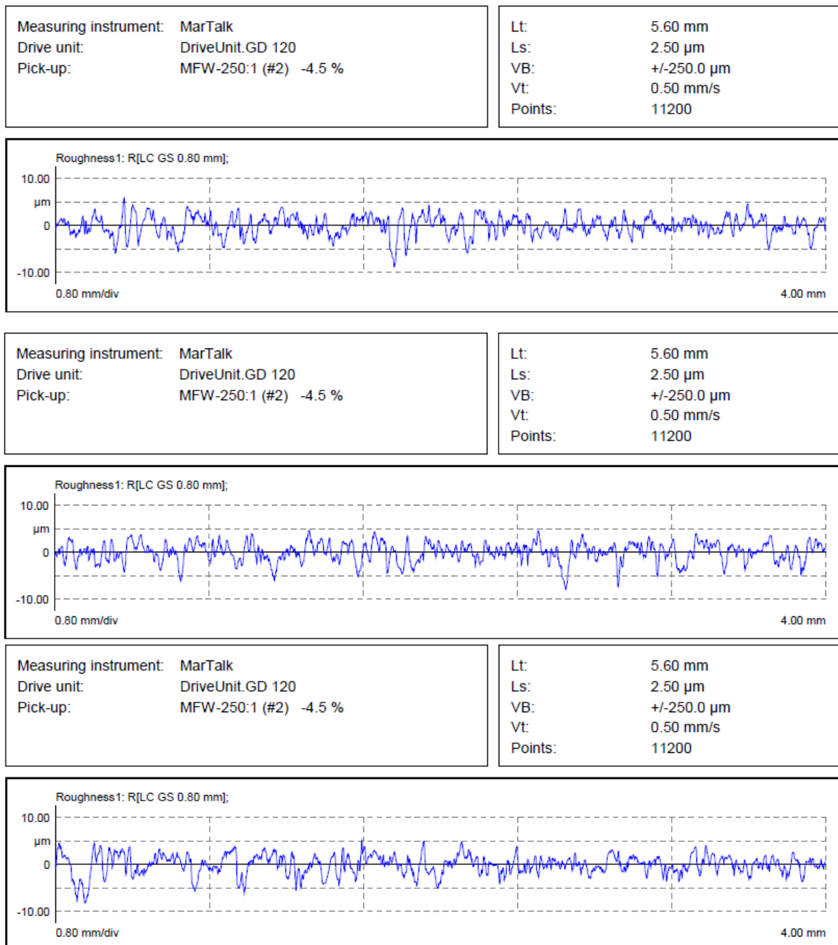
Figure 3. Surface profilometer study on the uncoated samples.
