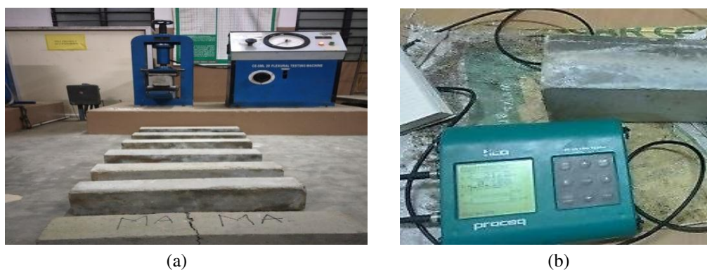
Figure 3 Specimen testing and UPV testing machine
