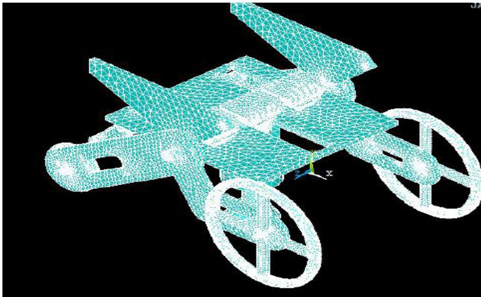
Fig.6. Meshed sequence of wheelchair
