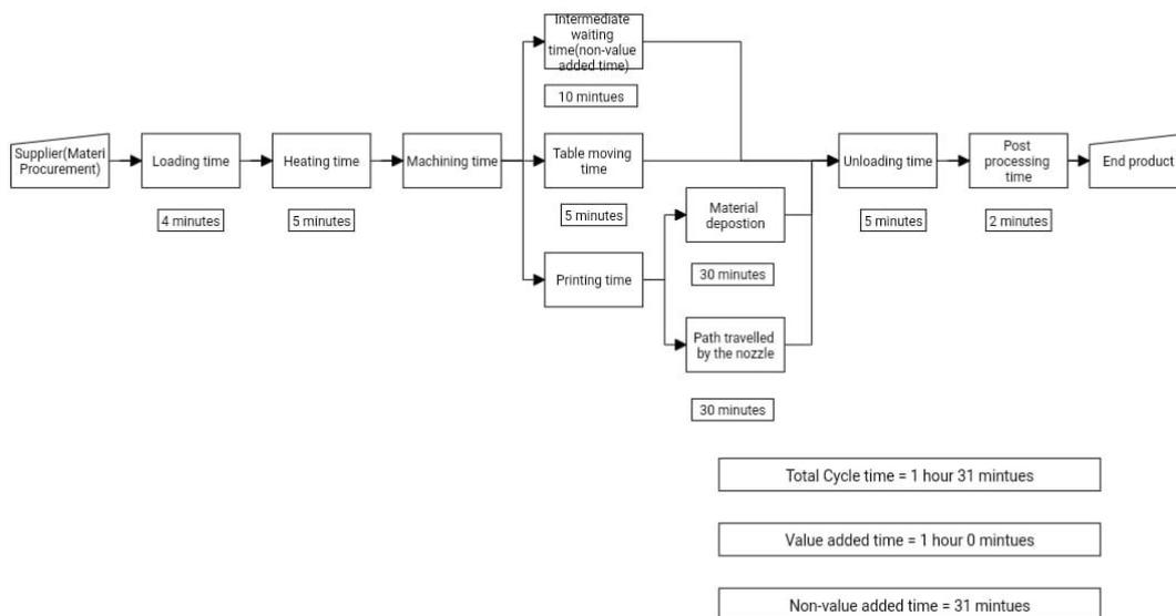
**Figure 8** VSM map for printing a sample model
