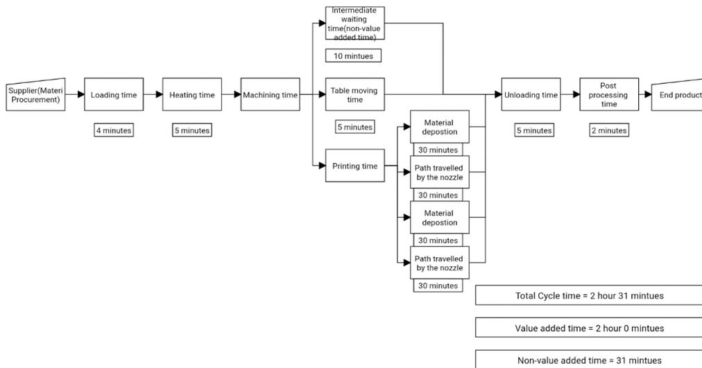
**Figure9** VSM map for printing grouped model simultaneously
