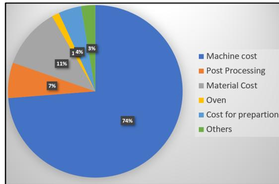
**Figure 1** Cost drivers pertaining to FDM process.
