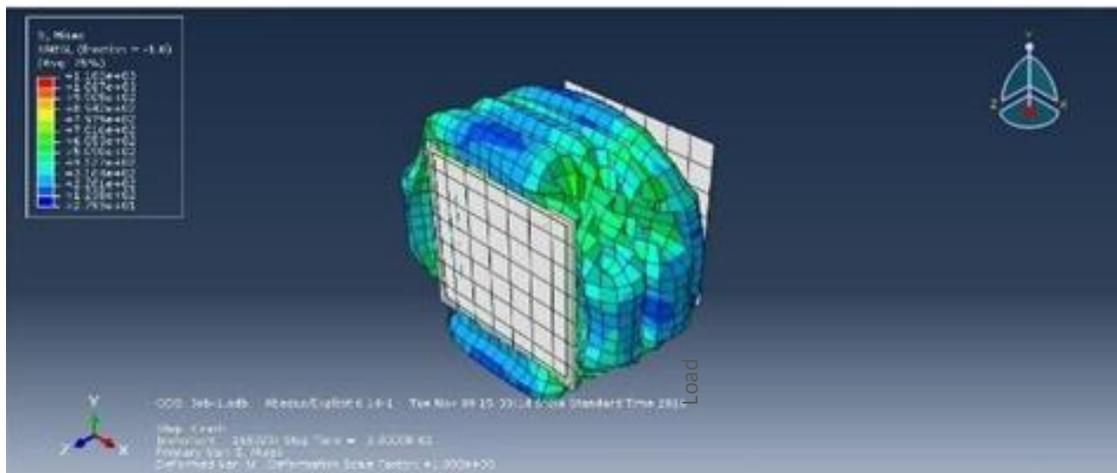
**Figure 8.**Crushed Al/CFRP [0/90]
