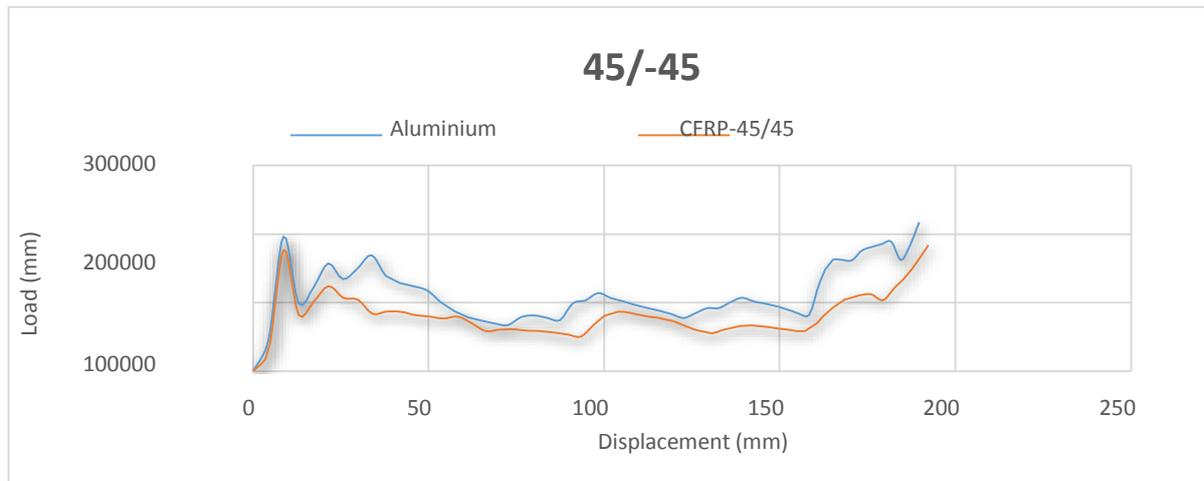
**Figure 11.** Load Displacement curve for [45/-45]
