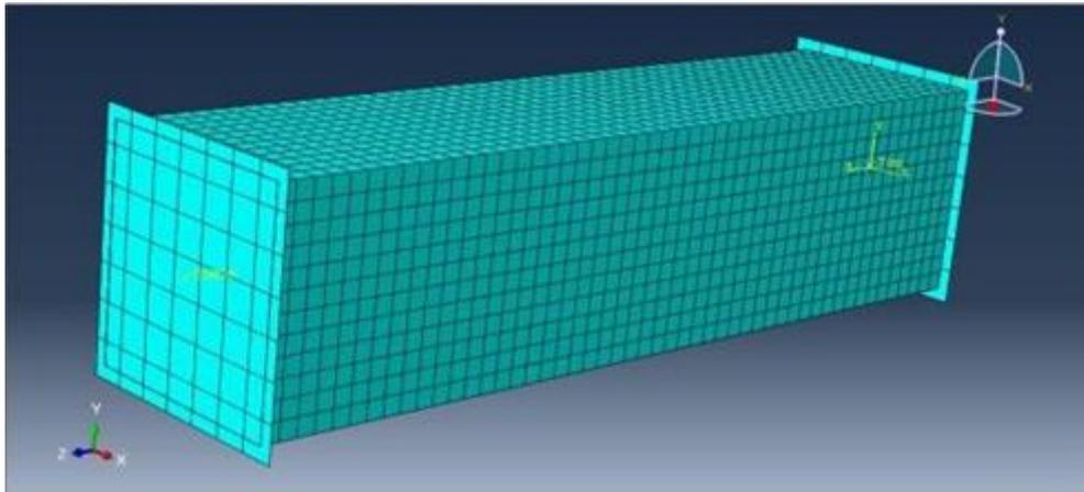
**Figure 1.** Meshed Hybrid beam in ABAQUS CAE
