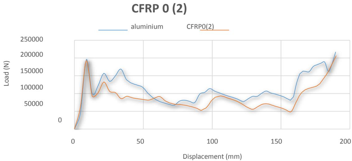
**Figure 5.** Load Displacement curve for  $[0]_2$
