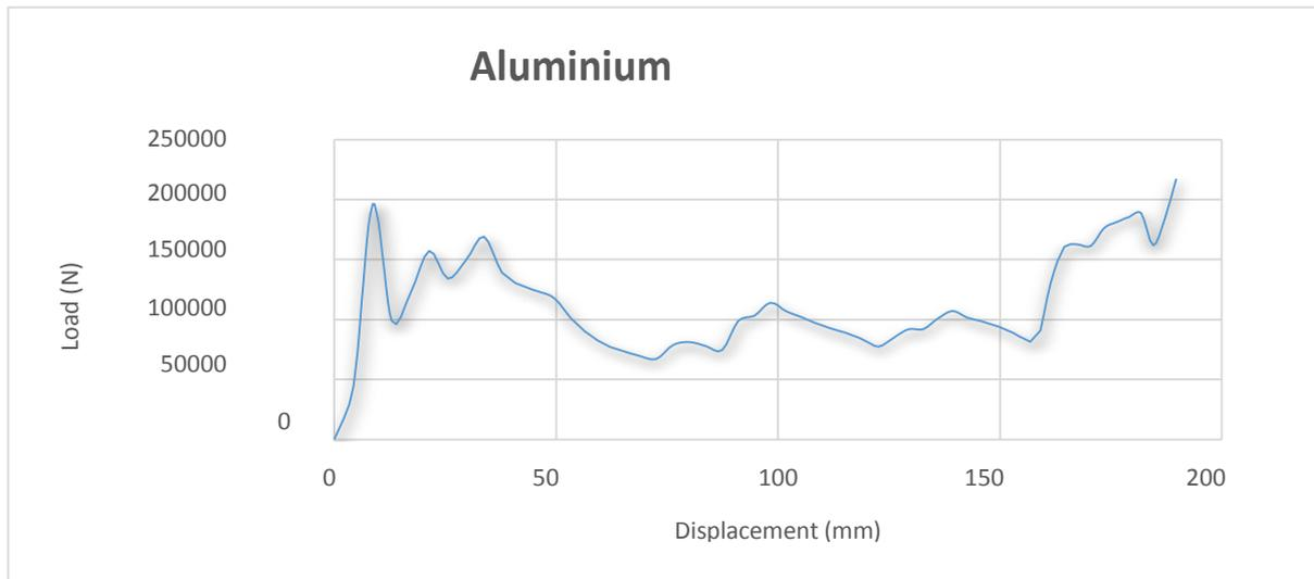
**Figure 3.** Load Displacement curve for Aluminium
