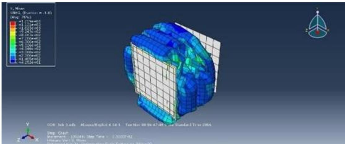
**Figure 10.** Crushed Al/CFRP  $[45^{\circ}/-45^{\circ}]$
