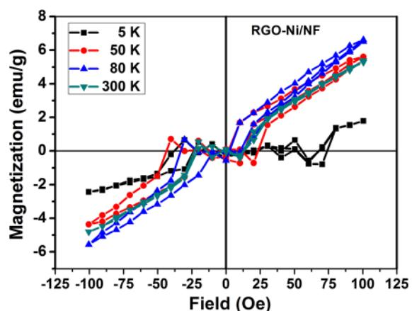
FIG. 5. M-H loops for RGO-Ni/NF nanocomposite at various temperatures.
