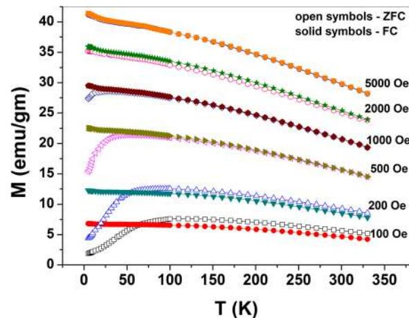
FIG. 4. ZFC-FC curves for RGO-Ni/NF nanocomposite.
