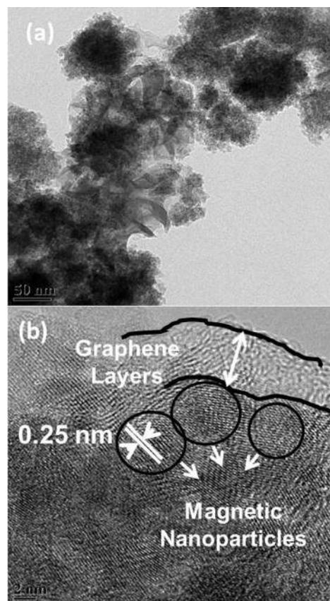
FIG. 2. HRTEM of RGO-Ni/NF nanocomposite at a scale of 50 nm (a) and 2 nm (b).
