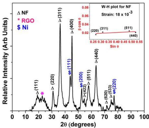
FIG. 1. XRD of RGO-Ni/NF nanocomposite.
