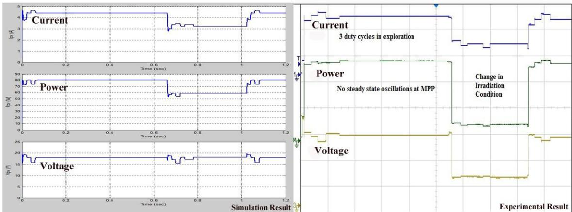
Fig. 3 Simulated and experimental results of voltage, current, and power tracked using modified PSO algorithm for variation in irradiation condition
