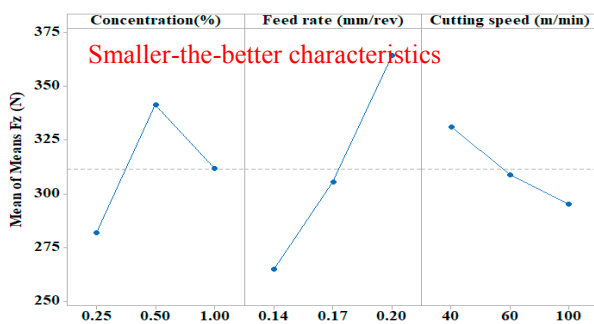
Fig. 3. Main effect plots for cutting force.
