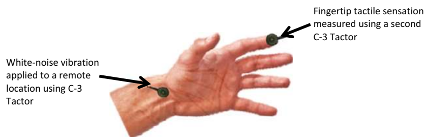
Figure 2. One vibrator (C-3 Tactor) was placed on a remote location (volar wrist in this figure) to provide white-noise suprathreshold (perceivable) or subthreshold (imperceptible) vibration, while a second vibrator was placed on the fingertip pad (the index fingertip in this figure) to measure the fingertip tactile sensation score.
