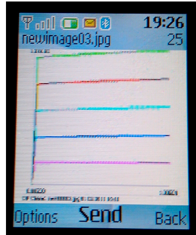
Figure 6. The output image of output characteristics of a BJT using WAP in Nokia 2630.
