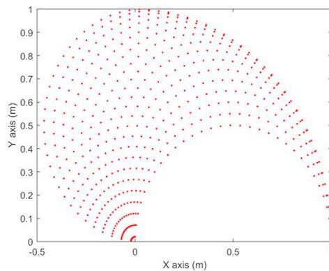
Fig. 4. Simulated workspace of 2R robot for the link length of  $l_1 = l_2 = 0.5\text{m}$ .
