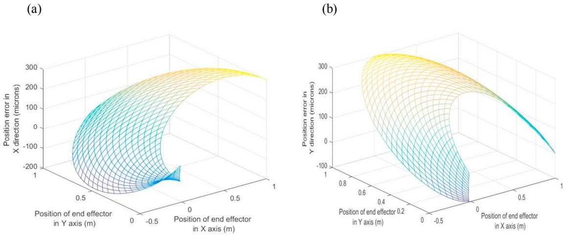
Fig. 5. (a) Position error of the end effector in X direction; (b) Position error of the end effector in Y direction.
