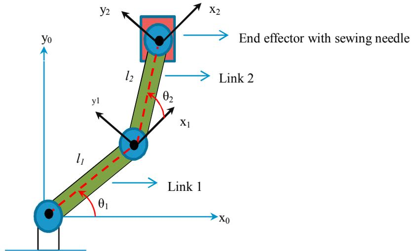
Fig. 1. Configuration of a 2R planar manipulator with D-H link parameters for sewing process.
