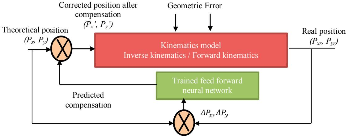
Fig. 2. Proposed methodology for position error correction using ANN in the robot manipulator.
