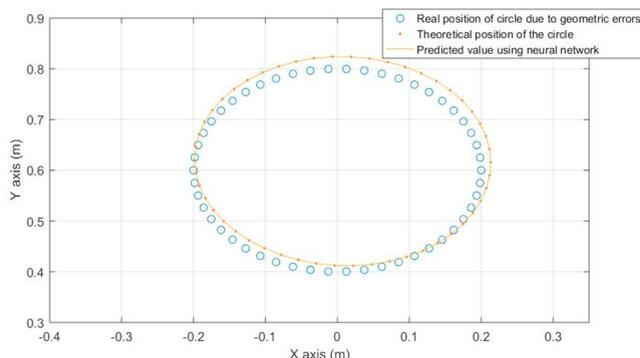
Fig.7. Simulation results of proposed approach for position error correction of circle.
