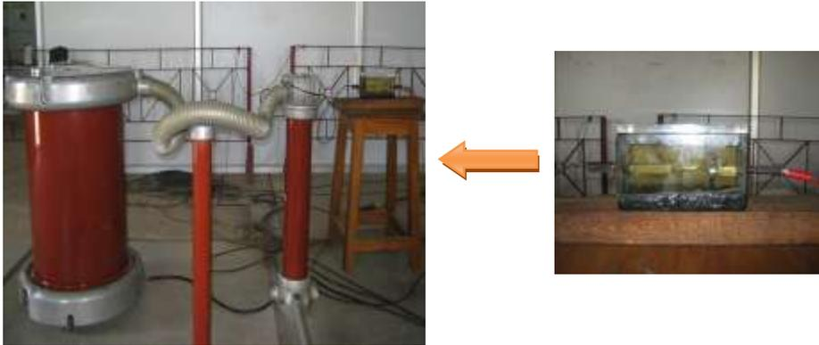
Figure. 2. Test Setup for PD Testing with oil test container.
