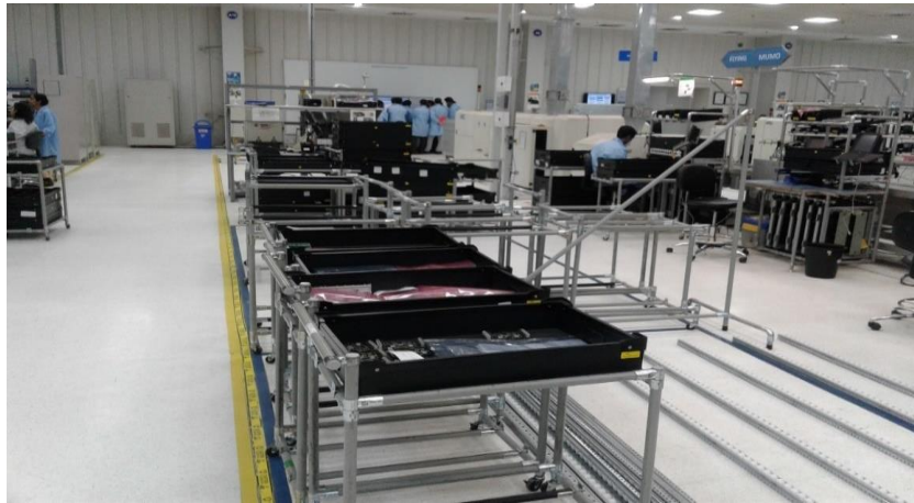
Figure 2. Bin trolley system for material transfer from THT to ICT line
