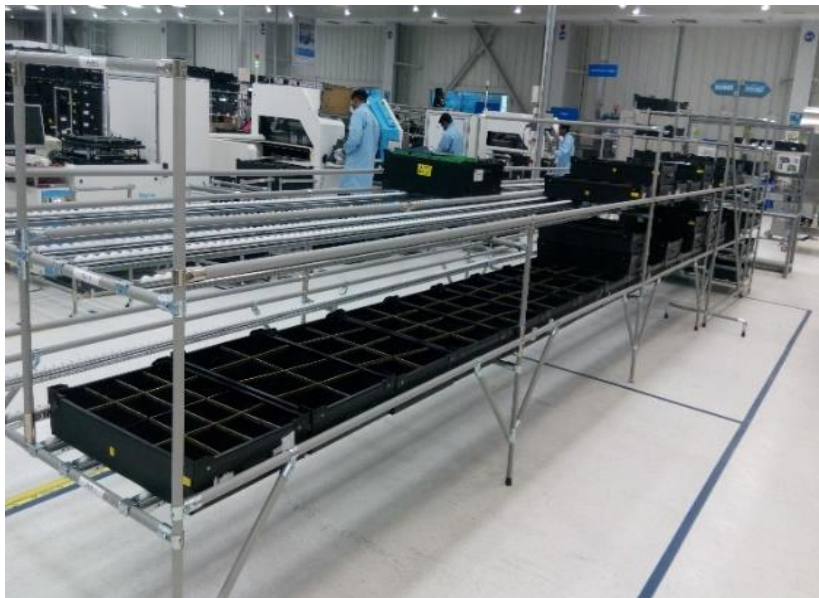
Figure 7. Prototype of conveyor developed on ground level for concept realization
