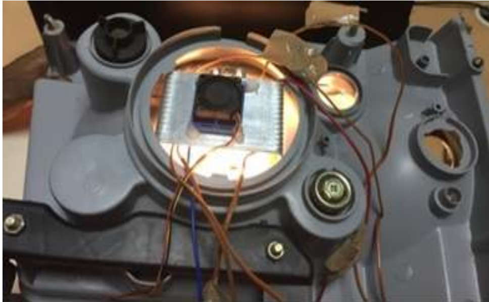
Figure 4. Headlamp assembly with heatsink and cooling fan
