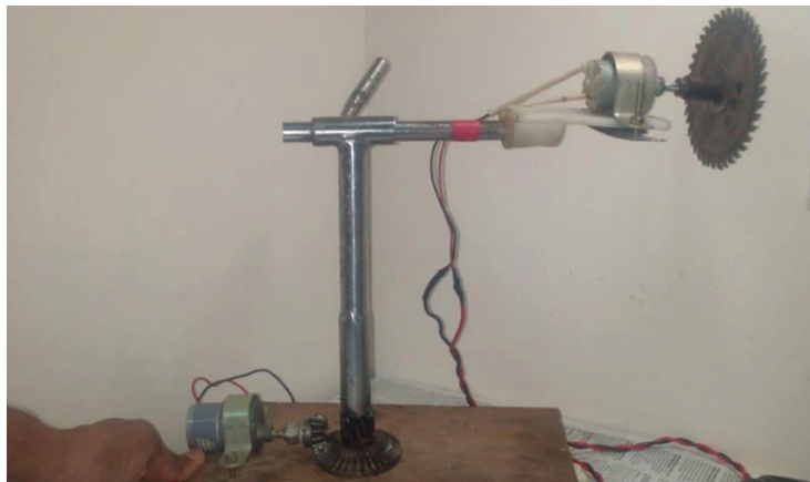
Fig.10.The arm with bevel gear arrangement and circular saw teeth blade for cutting
