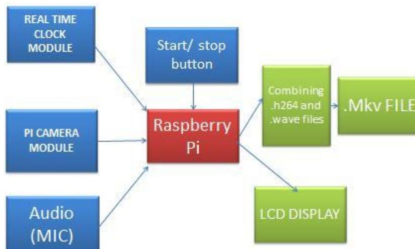
**Figure 1.** Block diagram of the body worn camera
