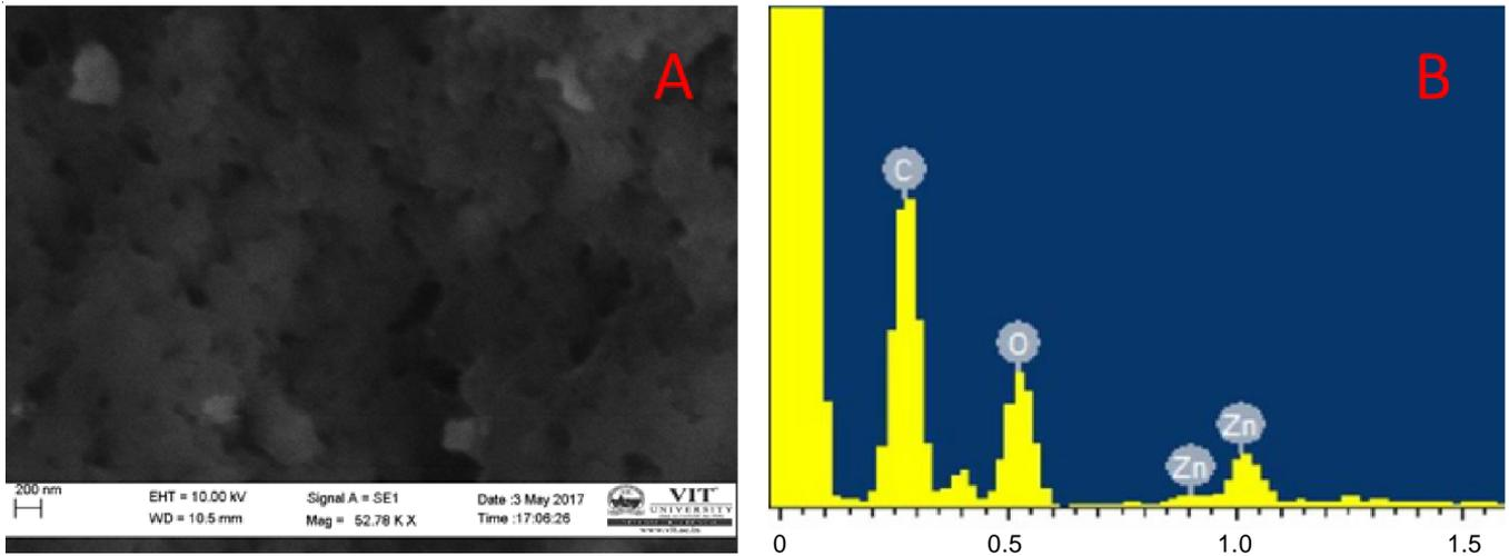
Fig. 3. (A) SEM micrograph of ZnO nanoparticle (B) EDAX of ZnO nanoparticle
