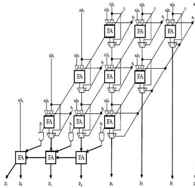
Fig. 3 4\*4 column bypassing
