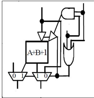
Fig.7 Row & Column Bypassing Adder Cell.
