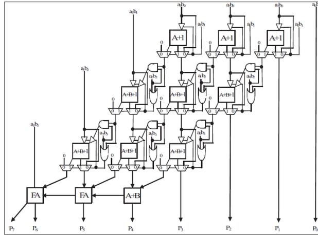
Fig. 6. Column and row bypassing multiplier
