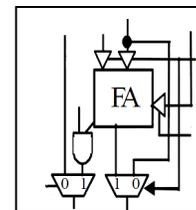
fig. 5. Adder cell
