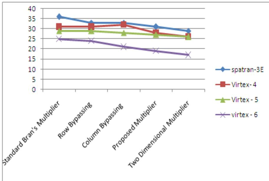
Fig. 8 The LUTs for Spartan-3AN, Virtex-4, Virtex - 5 and Virtex-6 for standard, row and column bypassing and proposed 4\*4 Braun's multipliers
