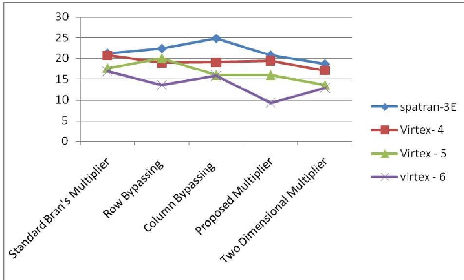
Fig. 11 The combinational path delay for Spartan-3AN, Virtex-4, Virtex - 5 and Virtex-6 for standard, row and column bypassing and proposed 4\*4 Braun's multipliers
