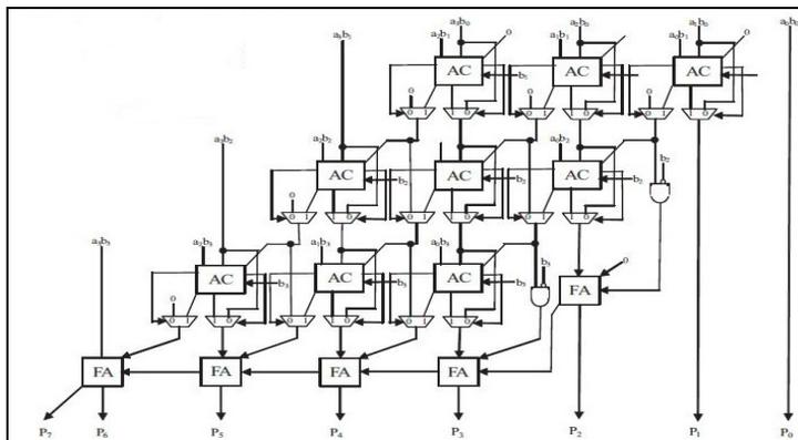
Fig 4. 4x4 2D Bypassing Multiplier in Braun Multiplier
