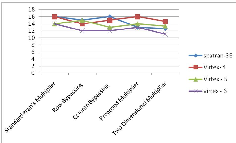
Fig. 10 The bonded IOBs for Spartan-3AN, Virtex-4, Virtex - 5 and Virtex-6 for standard, row and column bypassing and proposed 4\*4 Braun's multipliers
