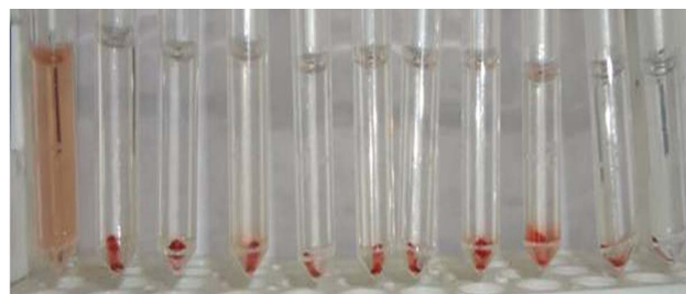
Figure 5. Hemolysis assay. The biocompatibility of ATV-BSA nanoparticles is shown with tubes from left to right as: PC-Positive control, NC-Negative Control, a to c, d to f and g to i showing the biocompatibility of 10, 15 & 20 \mu\text{g}/\text{mL} concentrations of ATV, BSA and ATV-BSA nanoparticles in RBC's respectively.
