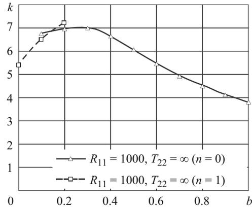
Fig. 8. Buckling load parameter  $k$  versus internal elastic ring support radius  $b$  for  $T_{22} = \infty, R_{11} = 1000$ .
