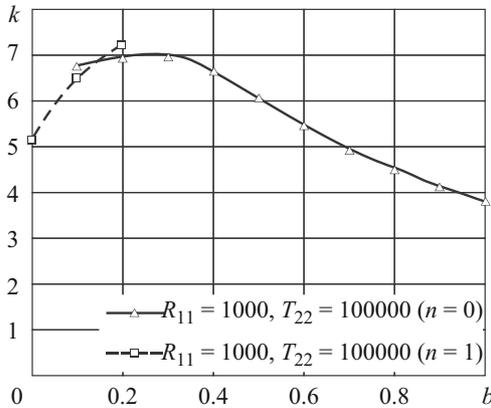
Fig. 7. Buckling load parameter  $k$  versus internal elastic ring support radius  $b$  for  $T_{22} = 100000, R_{11} = 1000$ .
