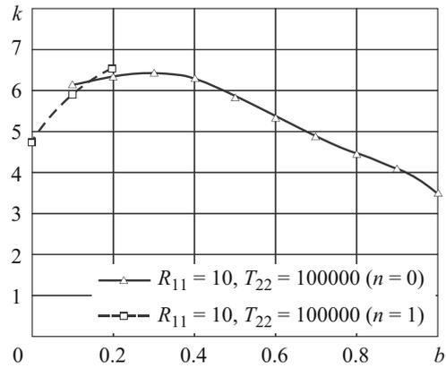
Fig. 3. Buckling load parameter  $k$  versus internal elastic ring support radius  $b$  for  $R_{11} = 10, T_{22} = 100000$ .
