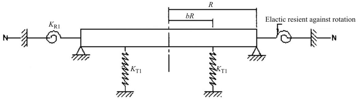
Fig. 1. Buckling of a circular plate with an internal elastic ring support and elastically restrained edge against rotation and simply supported.
