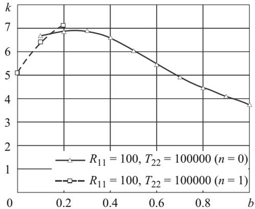
Fig. 4. Buckling load parameter  $k$  versus internal elastic ring support radius  $b$  for  $R_{11} = 100, T_{22} = 100000$ .
