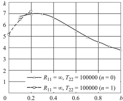
Fig. 5. Buckling load parameter  $k$  versus internal elastic ring support radius  $b$  for  $R_{11} = \infty, T_{22} = 100000$ .
