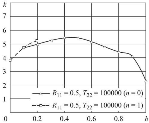
Fig. 2. Buckling load parameter  $k$  versus internal elastic ring support radius  $b$  for  $R_{11} = 0.5, T_{22} = 100000$ .
