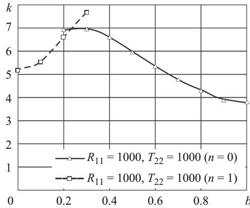
Fig. 6. Buckling load parameter  $k$  versus internal elastic ring support radius  $b$  for  $T_{22} = 1000, R_{11} = 1000$ .
