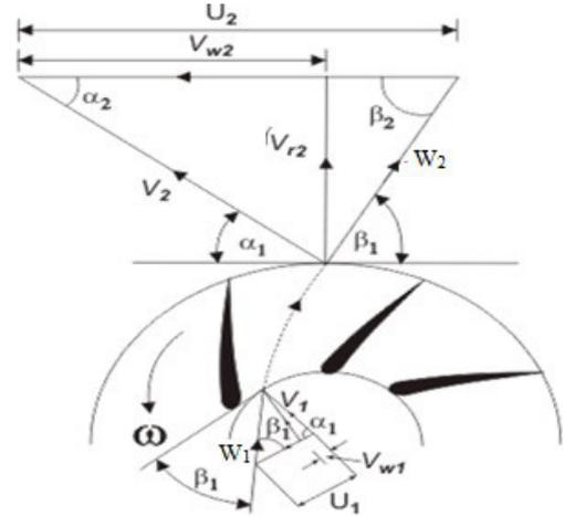
Fig. 4 Inlet and outlet velocity triangle
