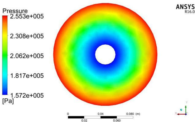
Fig. 14 Pressure distribution in original casing
