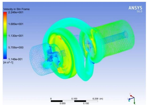
Fig. 17 Vector plot of velocity distribution in casing
