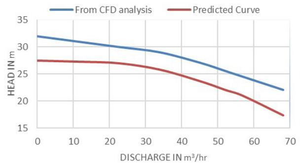
**Fig. 19** Head vs. Discharge
