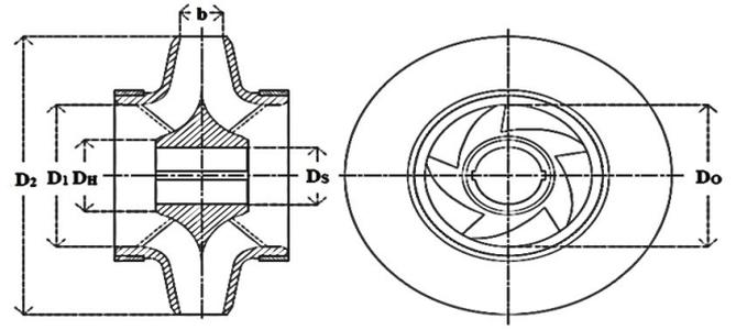
Fig. 3 Parameters of suction impeller
