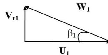
Fig. 1 Inlet velocity triangle
