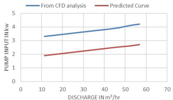
**Fig. 21** Pump Input vs. Discharge
