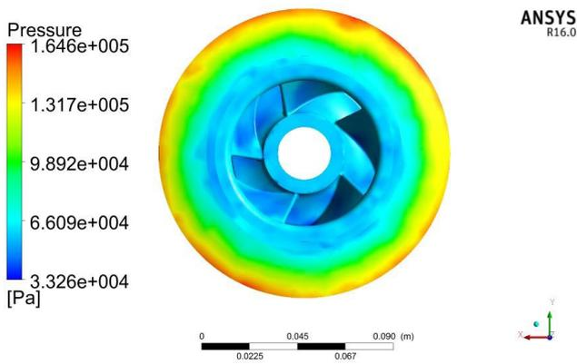
Fig. 13 Pressure distribution plot of impeller
