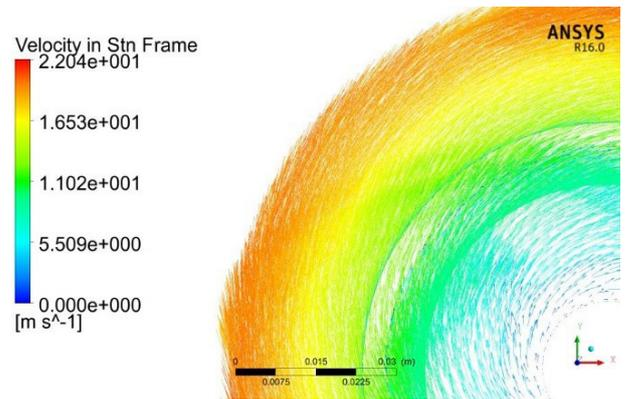
Fig. 15 Vector plot of velocity distribution in impeller
