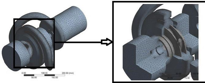
Fig. 12 Meshing of model
