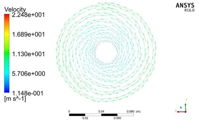
Fig. 16 Velocity Distribution in Original Casing
