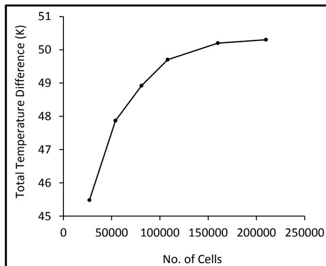
**Figure 3.** Grid independence study on Total temperature difference.
