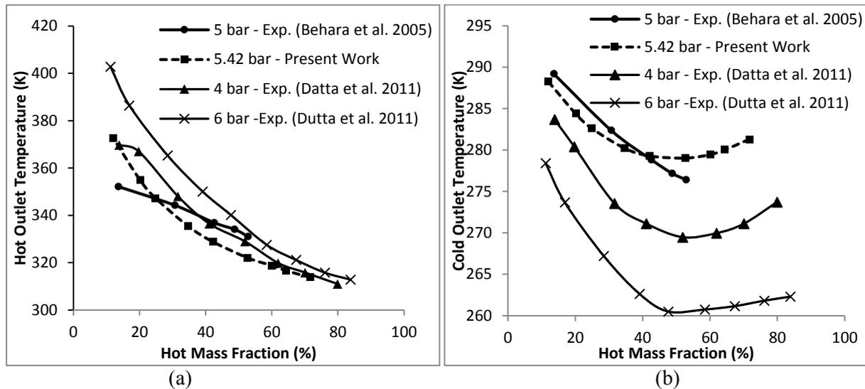
**Figure 4.** Comparison of experimental and CFD results.
