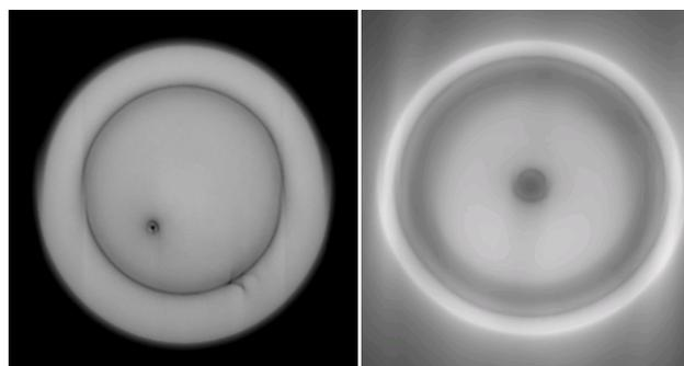
**Figure 3:** a) reconstructed image of the capillary b) reconstructed image of the finger phantom using FDK based reconstruction software
