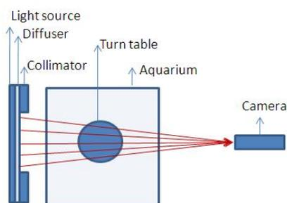
**Figure 1:** Schematic representation of the Optical Scanner.
