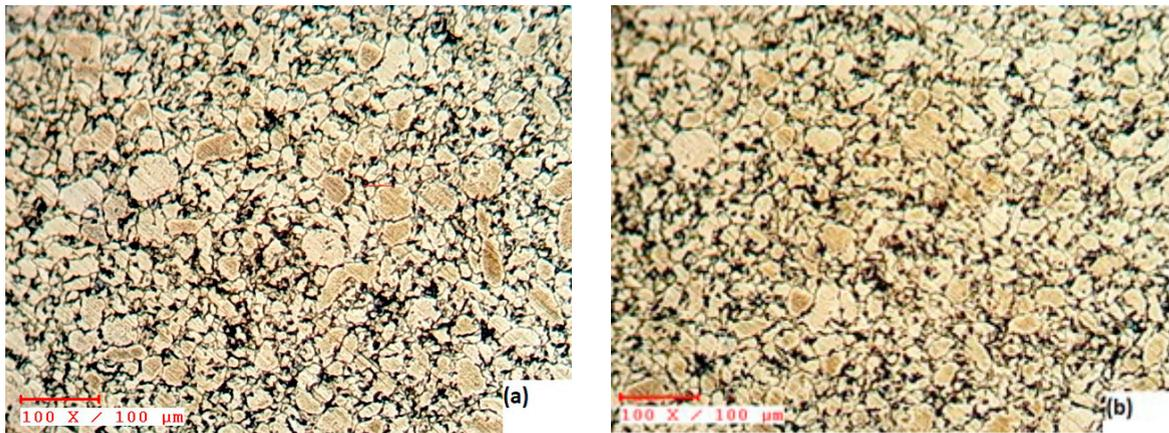
Fig. 1 SEM images of (a) Stir cast (b) Squeeze casting of AA7050-graphene composite material
