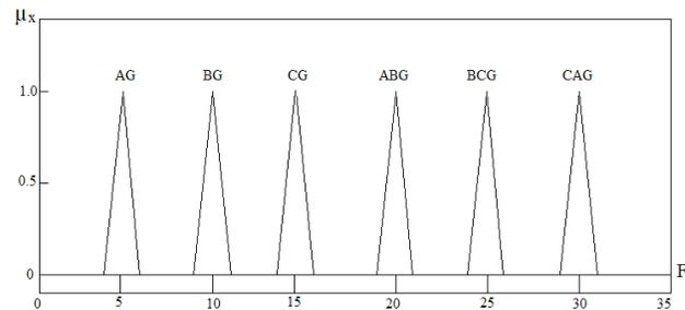
Figure 5. Triangular membership functions for outputs.
