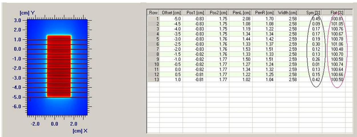
Fig. 2 – Flatness and symmetry results from film dosimetry.
