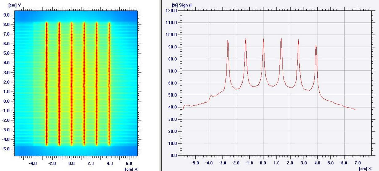
**Fig. 10** – The image obtained for the picket fence test with a sub millimeter error introduced taken on EDR2 therapy film. The planned error is exactly observed in the image.
