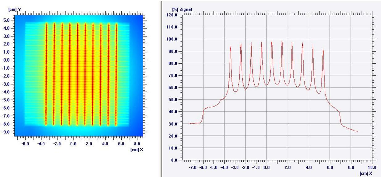
Fig. 7 – The image obtained for the picket fence test at a stationary angle and during gantry rotation on a EDR2 therapy film.
