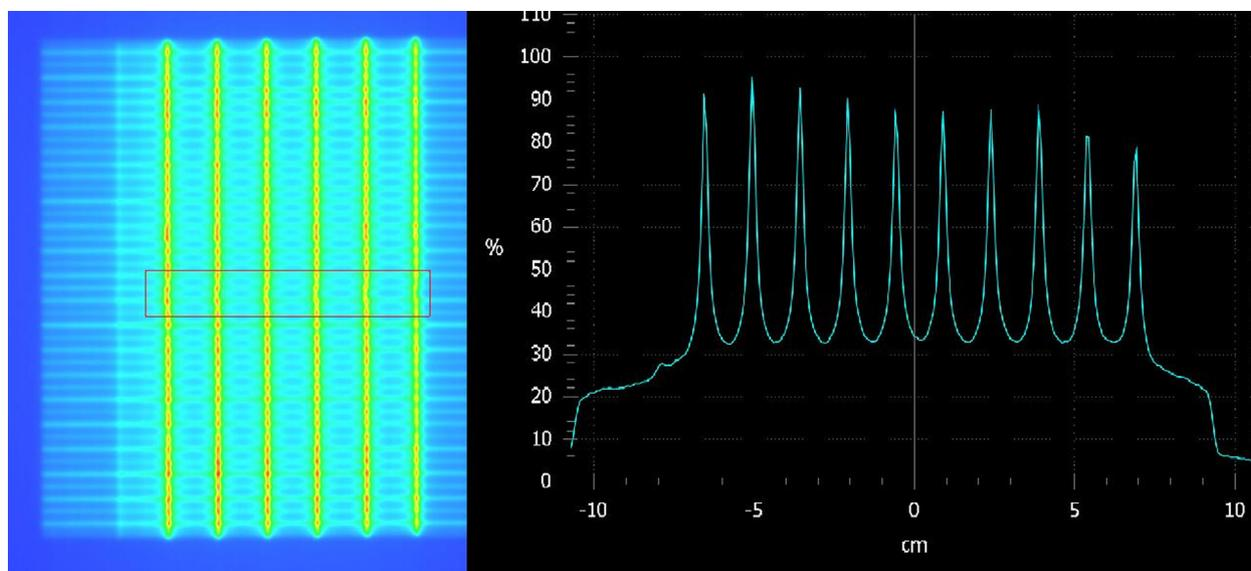
**Fig. 11 – The image obtained for the picket fence test with a sub millimeter error introduced taken on EPID and evaluated using the Portal Dose Prediction Software. As seen above the portal dose image also shows the sub millimeter error introduced in the MLC position.**
