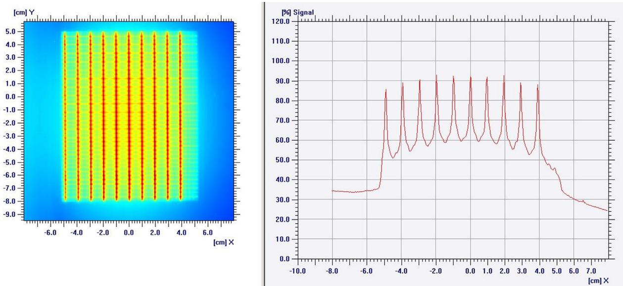
Fig. 5 – The image obtained for the picket fence test at a stationary angle on a EDR2 therapy film.
