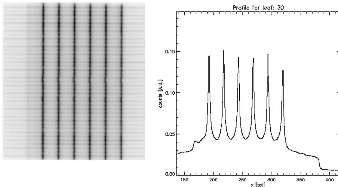
**Fig. 12 – The image obtained for the picket fence test with a sub millimeter error introduced taken on EPID and evaluated using the EPIQA. Intentional errors introduced in the picket fence pattern were clearly noticeable.**
