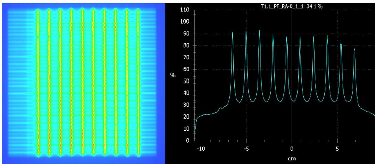
Fig. 8 – The image obtained for the picket fence test at a stationary angle and during gantry rotation on EPID and evaluated using the Portal Dose Prediction Software.
