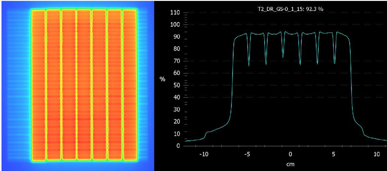
**Fig. 14 – The image taken on EPID and evaluated using the Portal Dose Prediction Software to evaluate accurate control of dose rate and gantry speed during RapidArc delivery. Even the portal dose shows equal exposures in all strips.**
