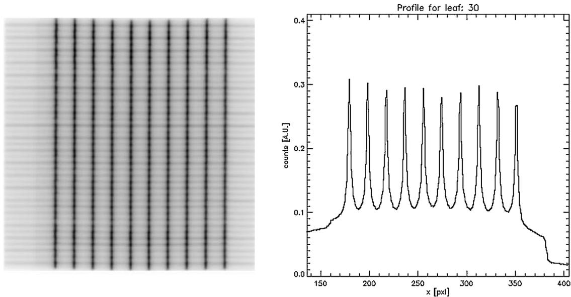
**Fig. 9** – The image obtained for the picket fence test at a stationary angle and during gantry rotation on EPID and evaluated using the EPIQA.
