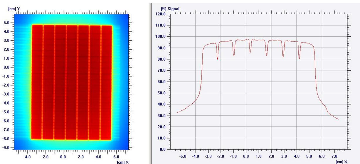
**Fig. 13 – The image taken on EDR2 therapy film to evaluate accurate control of dose rate and gantry speed during RapidArc delivery. All the strips show equally exposed regions when evaluated with Omnipro software.**
