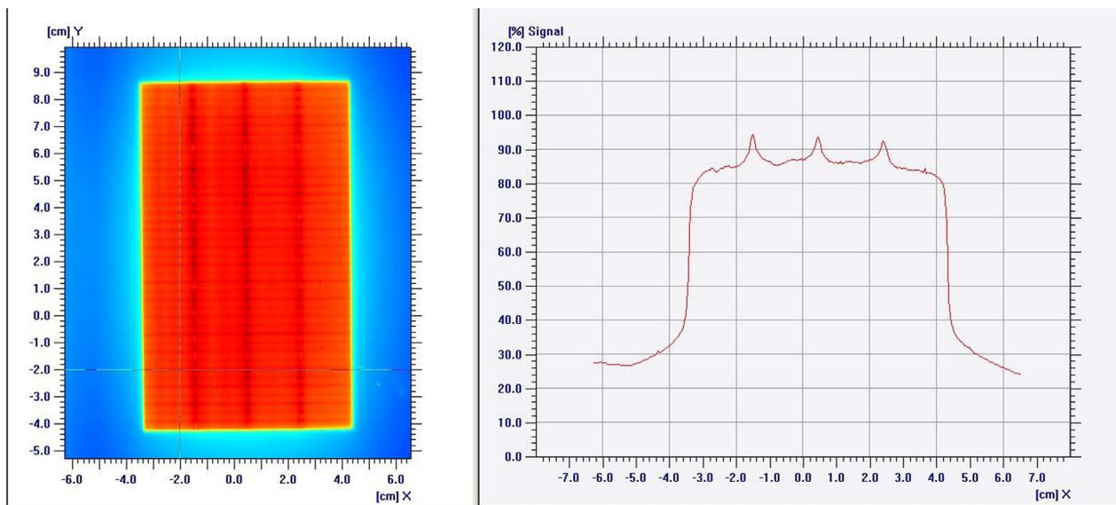
**Fig. 15 – The image obtained on EDR2 therapy film to evaluate accurate control of leaf speed during RapidArc delivery.**
