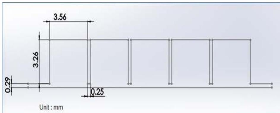
Fig. 1. Dimensions of labyrinth seal
