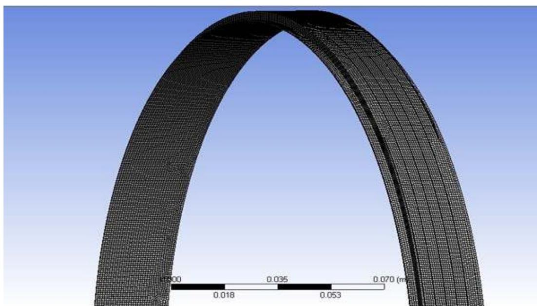
Fig. 4. Meshing of the model
