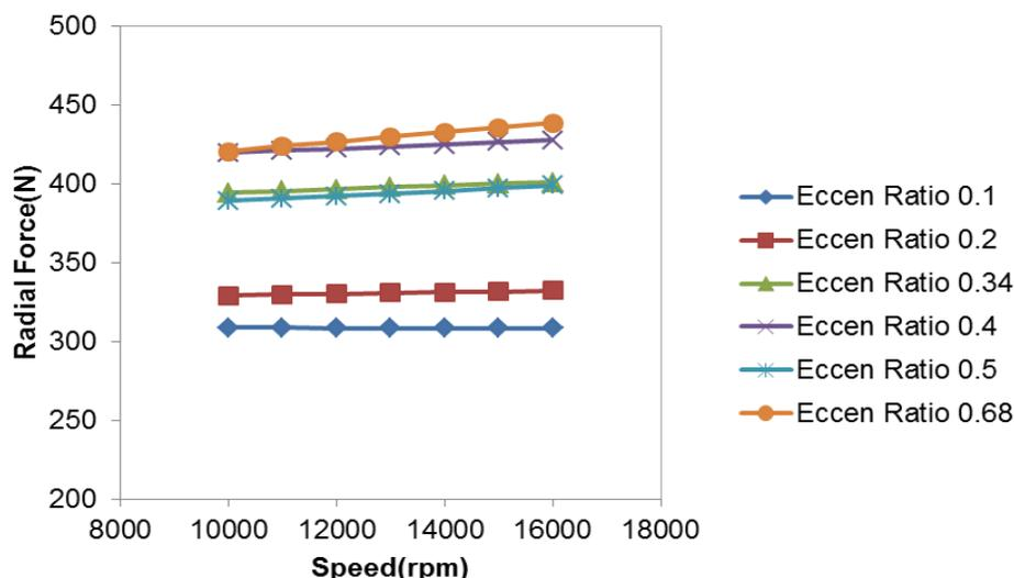
Fig. 8. Radial forces vs speed for helically-grooved labyrinth seal
