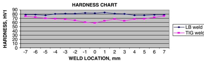
**Figure 5.** Hardness chart for TIG welding and LB welding.
