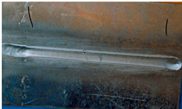
**Figure 1.** Bead appearance of TIG welding.
