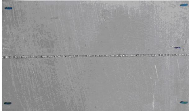
**Figure 2.** Bead appearance of LB welding.
