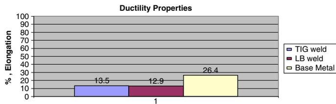
**Figure 4.** Ductility chart for TIG welding and LB welding.
