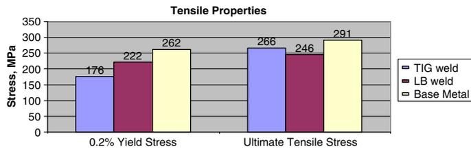
**Figure 3.** Tensile properties of TIG welding and Laser beam welding.
