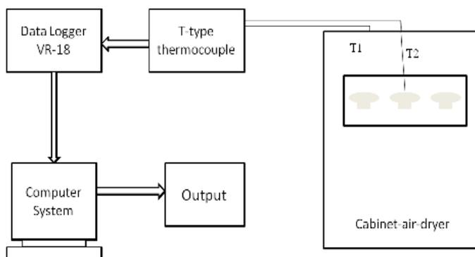
Figure 1 Schematic arrangement of the experimental setup.
