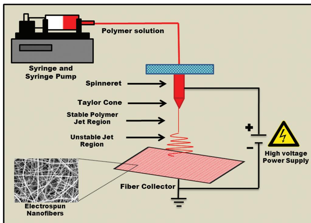
**Figure 1.** Schematic illustration of the electrospinning setup and process conditions.
