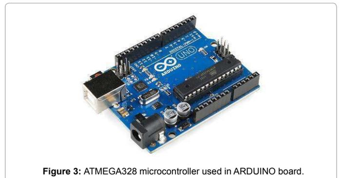
Figure 3: ATMEGA328 microcontroller used in ARDUINO board.
