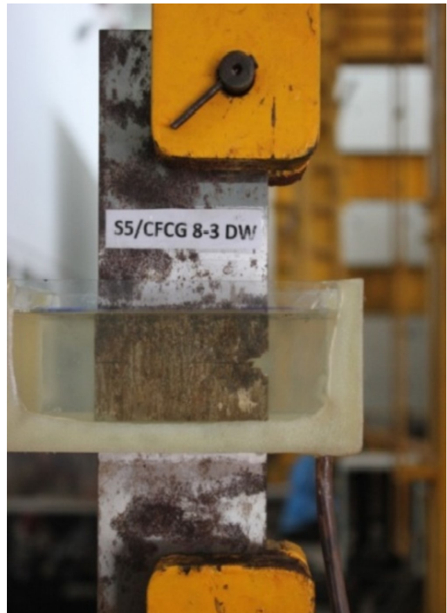
Fig. 3. Close-up view of the ESE(T) specimen and corrosion chamber
