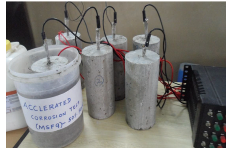
FIGURE 3: Snapshot for concrete specimens immersed in 3.5% sodium chloride solution.
