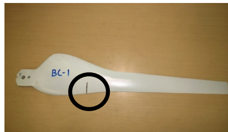
Figure 3b: Blade root crack fault
