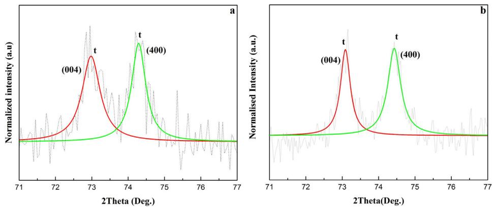
**Fig. 10 – Deconvoluted (Lorentzian fit) XRD pattern of annealed 4Gd4SmSZ powders at 1573 K for 10 h b) 100 h showing tetragonal phase.**
