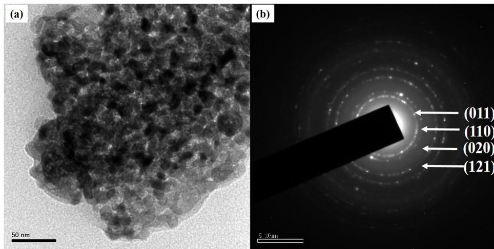
**Fig. 8 – HR-TEM of 4Gd4SmSZ powders a) bright field image b) Selected Area Electron Diffraction pattern.**
