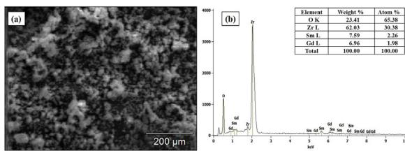
**Fig. 7 – SEM micrograph of a) 4Gd4SmSZ powders calcined at 1073 K b) Energy-dispersive spectra showing the corresponding constituents.**
