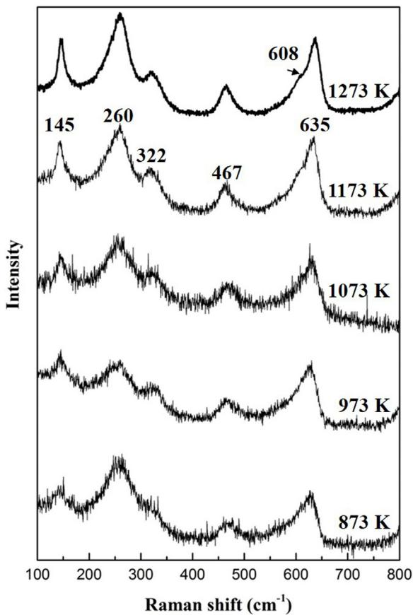
Fig. 4 – Raman spectra of 4Gd4SmSZ powders at various temperatures.
