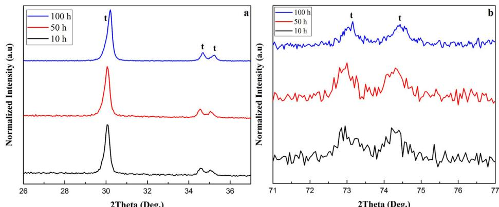
**Fig. 9 – XRD pattern of 4Gd4SmSZ powders annealed at 1573 K a) low angle region b) high angle region.**
