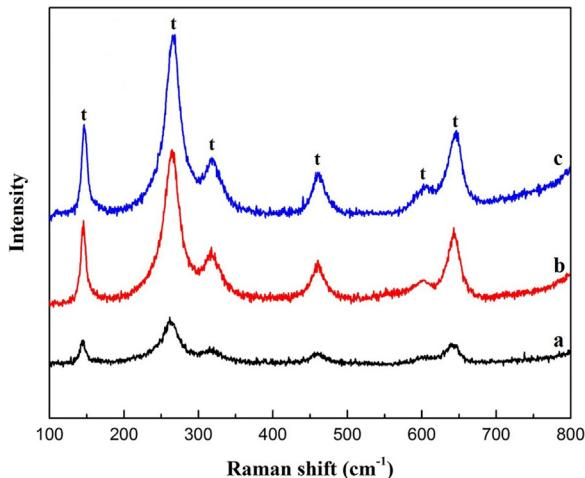
**Fig. 11 – Raman spectra of annealed 4Gd4SmSZ powders at 1573 K for a) 100 h, b) 50 h, and c) 10 h.**
