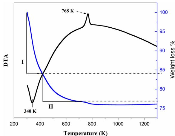
Fig. 1 – TG-DTA curve of 4Gd4SmSZ powders.
