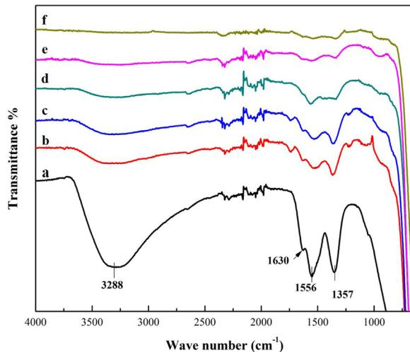
**Fig. 2 – FTIR spectra of 4Gd4SmSZ powders a) as prepared b) 873 K c) 973 K d) 1073 K e) 1173 K and f) 1273 K.**
