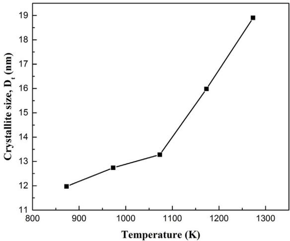
Fig. 5 – The evolution of crystallite size versus calcination temperature of 4Gd4SmSZ powders.
