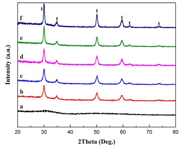
**Fig. 3 – XRD pattern of 4Gd4SmSZ powders a)573 K b) 873 K c) 973 K d)1073 K e) 1173 K and f) 1273 K.**
